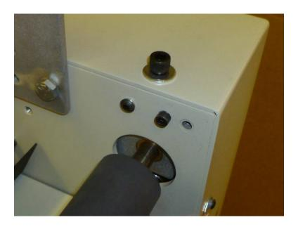
3. Using the #10 flat head screw install the screw through the tapered hole in the bracket and screw into position #8. Make sure that the bracket sits flat and flush against the panel and tighten securely.
